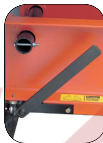
Lever lowers bed for pressing, raises it for rolling.
